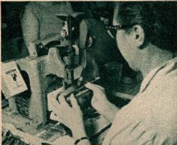
ABOVE: The front and rear brushes of the Model Motoring cars are aligned and then riveted to the chassis by this machine.
