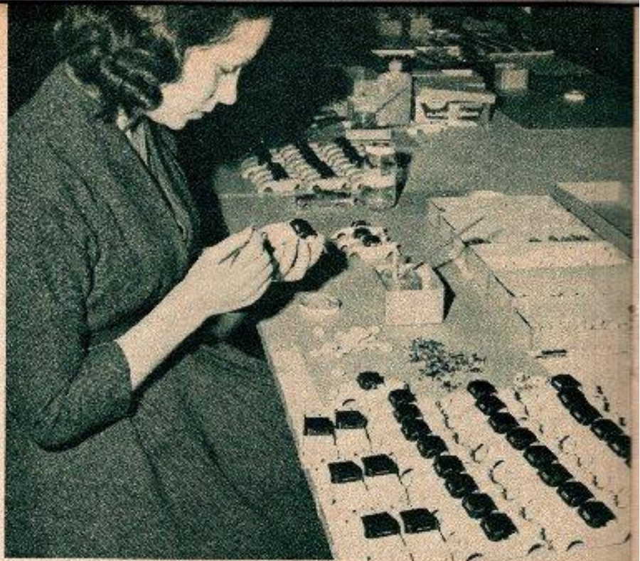
BELOW: This young lady is assembling one of the unique features of the Model Motoring test, a mechanical lap counting device.
