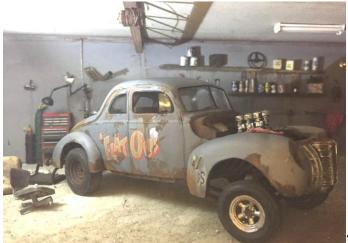
40 Ford gasser based on the 1/25-scale Lindberg kit, with straight axle from the Malco gasser kit and 3D-printed rear "steelies."
