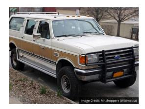
The Centurion Classic was produced from 1987 until 1996 when the Bronco was dropped by Ford. There were two models of Centurion Classic: The C150 and the C350, which used an F-150 and an F-350 respectively. Regardless of which model F-series was used, it needed to be the Crew Cab configuration in order to provide the additional interior space that was needed.
